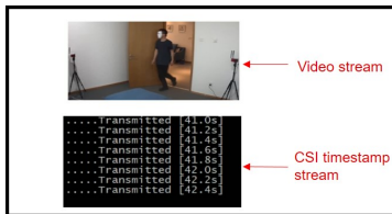
Fig. 14. An example frame of auxiliary video for synchronization
